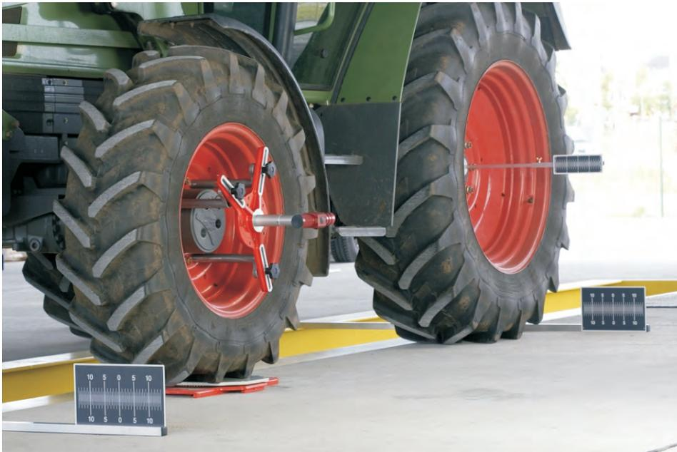
Laser wheel alignment system for tractors and agricultural machinery
