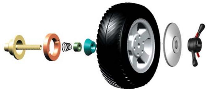
Both clamping hoods have rubber rings that are fitted to the contact surface. These work well with the alloy wheels but create problems when used on steel wheels.
